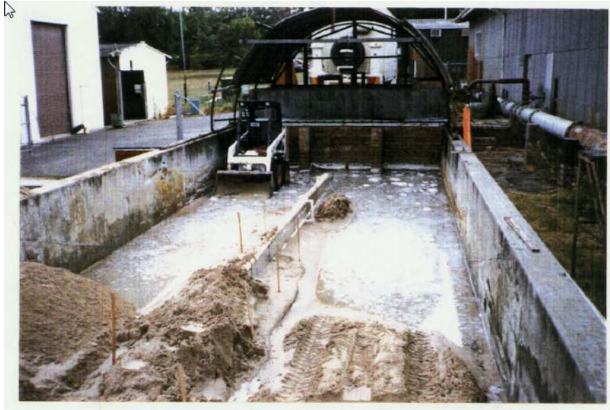
Figure 6 Photo of pilot scale shifter in test basin partly covered with sand
